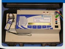
Portable measurement unit is a compact version of the DCtest2 system which includes a pulse generator and portable measurement clamp. This solution is especially recommended for users who have a few plants with relatively small DC networks, in case when they are not ready to install a stationary system on each plant.
